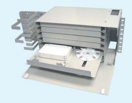
MFM Fiber Distribution Panels are designed for terminating optical fiber in exchanges or communications room where higher density is required. MFM features a modular system for fiber splicing and patching with flexible cable management systems. MFM consists of a splice module and a patch module to provide a cost effective and easy installation solutions for fiber optic management system.
